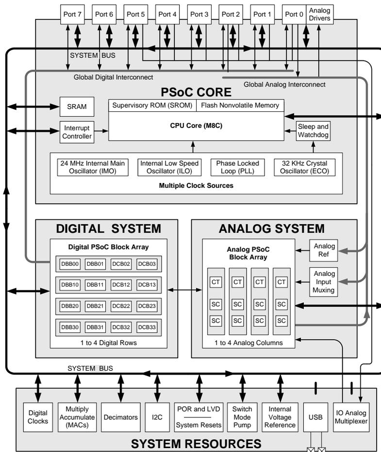
The analog PSoC block array is the focus of this application note. It consists of two basic analog blocks known as continuous time (CT) and switch capacitor (SC). Due to the configuration flexibility of these blocks, all the analog user modules, such as ADCs, DACs, and PGAs, available in PSoC Designer are created using these two basic blocks. The analog user modules created with these blocks include several ADCs, DACs, filters, mixers, PGAs, and other components.
