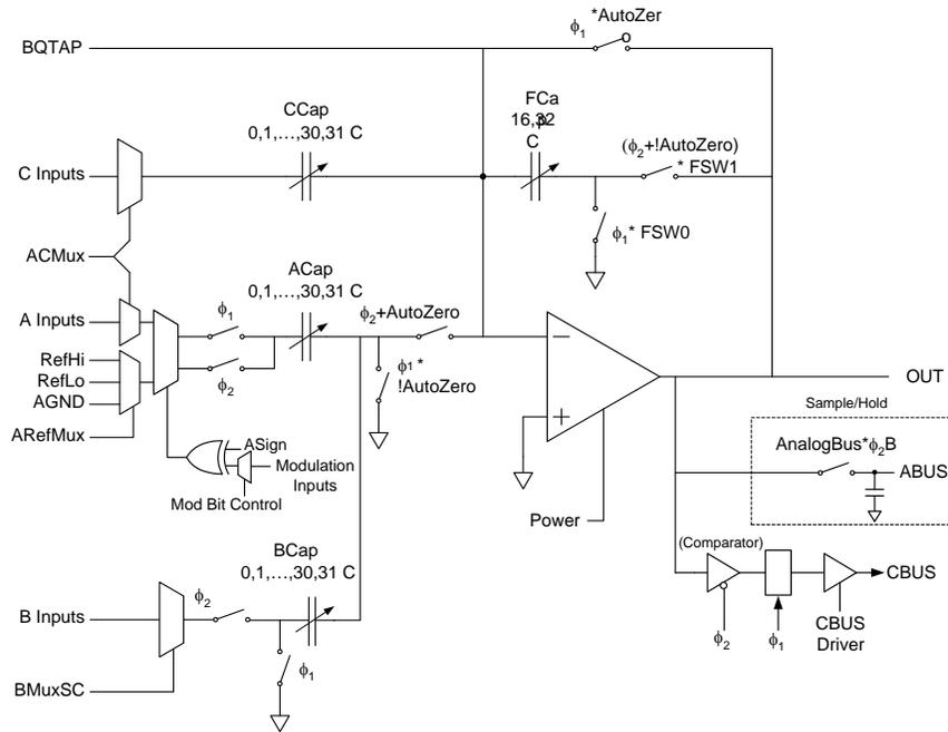
**Figure 7. PSoC 1 SC Type D Block**
