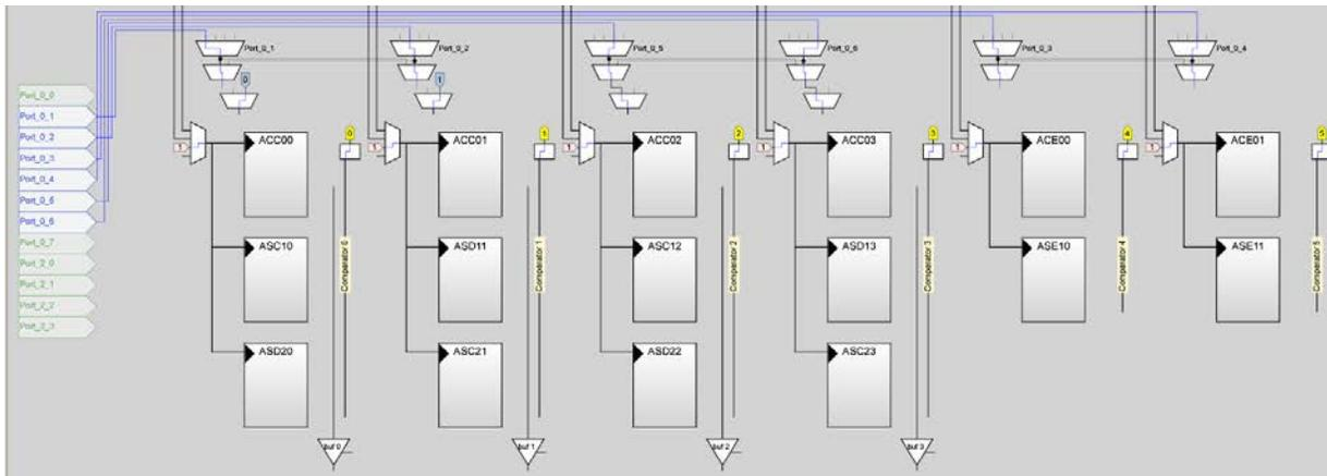
You may configure initial analog routes in PSoC Designer during design. They will be configured prior to user code execution (*main.c*). For applications in which some or all analog routes don't need to change during runtime, you do not need to generate additional code.
