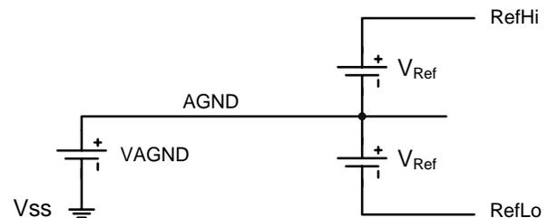
A simplified schematic of the reference (AGND, RefHi, RefLo) generation circuit is shown Figure 21.
