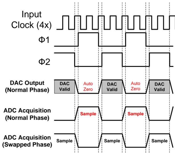
Looking at the “DAC Output” waveform in Figure 12, you may become concerned that the DAC output does not look like a continuous signal. Internally an SC block output will switch between its auto-zero and valid phase, but as long as the SC blocks are synced properly, this is not a problem. When routing the signal to the analog column bus, it passed through a sample and hold circuit. Each analog column has its own sample and hold, which convert the SC block output back to a continuous time signal.
