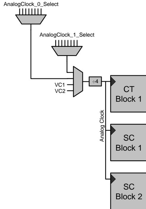
When analog signals are routed between blocks in adjacent columns, the clocks in these columns should be synchronized in phase and frequency. Frequency synchronization may be achieved by selecting the same input clock source for the columns.
