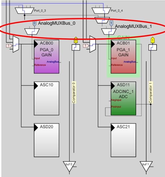
**Figure 16. AnalogMUXBus Connectivity**
