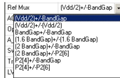
Analog voltage measurement and signal processing applications in PSoC 1 require the use of a precision ground and voltage references. Selecting the correct analog ground and voltage reference is essential in establishing accurate system performance. PSoC 1 offers considerable flexibility in setting references.
