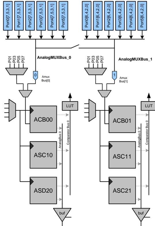
The CY8C24x8x parts have two AnalogMUXBuses that may be used independently or combined together. The Odd port pins may connect to AnalogMUXBus\_0 and the even pins can be connected to AnalogMUXBus\_1. These buses may be used to route any analog signal to one of the analog columns, or be used for CapSense in the parts that support it. Figure 16 shows port pins that can connect to each of the buses.
